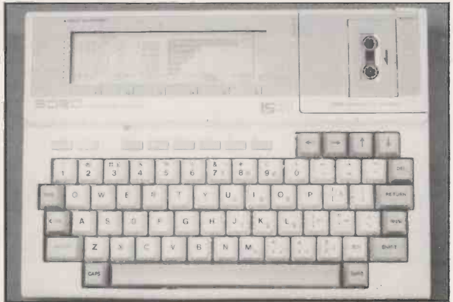
The IS-11 packs full-size keyboard, LCD display and microcassette drive into a compact A4 size battery-powered unit.
