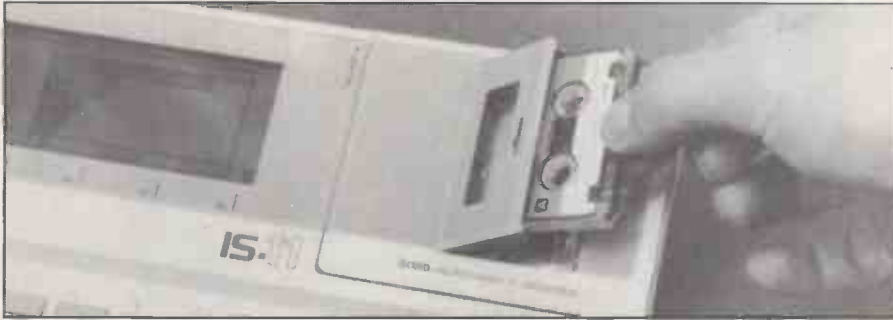
The built-in microcassette drive can store 128K of data on a standard dictation-machine-style C-30 cassette.
