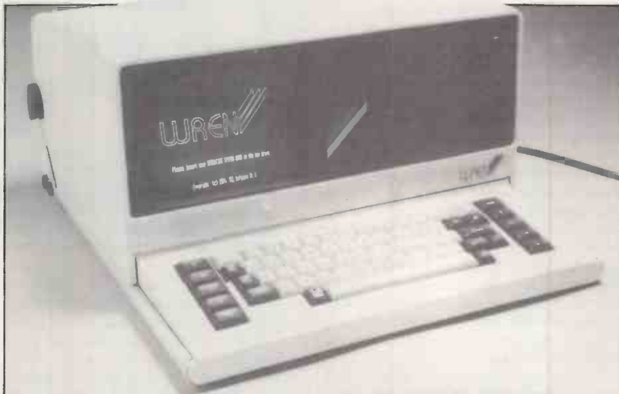
The combined screen and disc unit slide back to reveal the Wren's keyboard.
